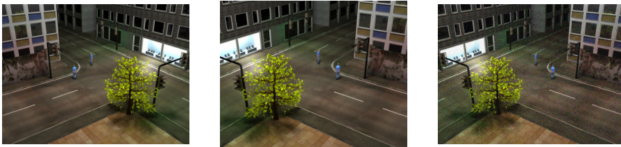
Plate 6. Default augmentation techniques (from left to right): image mirroring, centre cropping and adding noise
