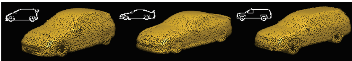
Figure 1: Examples of 3D car shapes generated by our system with side-view sketches.
