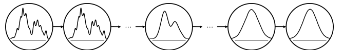
Fig. 2. The forward process perturbs the original unknown distribution by gradually adding noise to a given set of data samples through a chain of distribution transitions with multiple time steps. Each time step of the chain is denoted by a circle.
