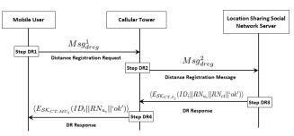
FIGURE 7: Message Communication in Distance Threshold Registration Phase refer to Section V-D.
