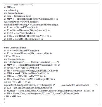
FIGURE 12: Code in ProVerif for the process of  $MU_i$ , the  $i^{th}$  mobile user
