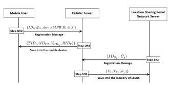
FIGURE 2: Message Communication in Registration Phase. Please refer to Sections V-A1 and V-A2.
