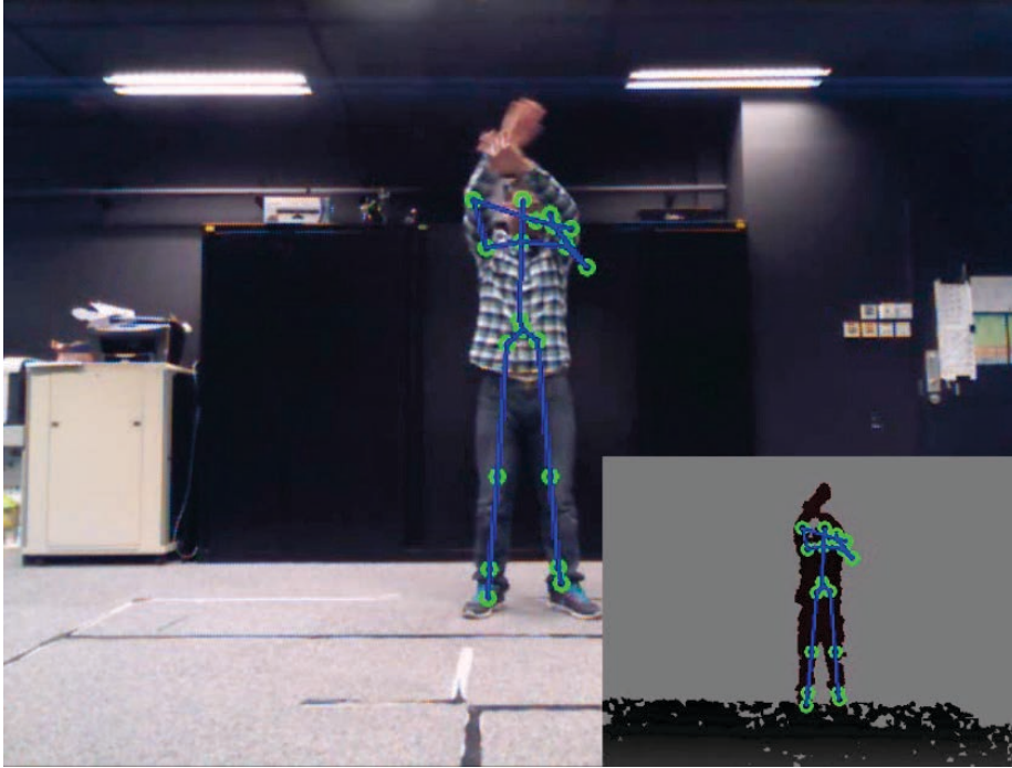
Figure 1.2: Example of an inaccurately tracked posture from Kinect. The blue skeleton is the tracked result by Kinect.
