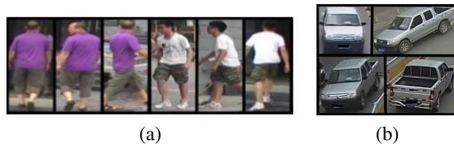
Figure 25: Matching people and vehicles contain different challenges: (a) Person shape and colour remains consistent across viewpoints; (b) Vehicle shape and colour changes drastically across viewpoints.
