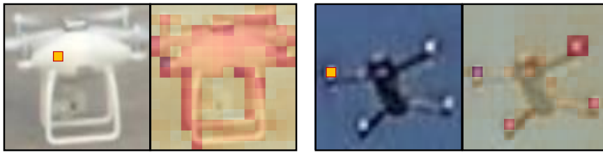
Figure 34: Attention visualisation of the transformer mechanism within ViT on the Big-to-Small setting. Attention from the 16 \times 16 yellow image patch is presented. Attention can highlight salient image patches relevant to the selected image patch.
